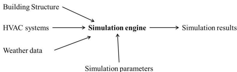
Figure 2: Input/output data of thermal simulation engines
