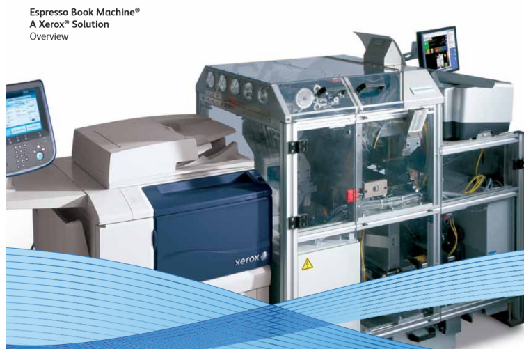
Figure 5.5. The Espresso Book Machine according to http://ondemandbooks.com
