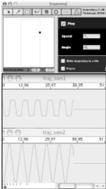
Figure 4. The coordinates of the rectangle trajectory on the top write themselves in the two buffers on the bottom. The upper buffer corresponds to the abscissa variation, the lower buffer to the ordinate variation.
